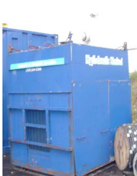
160 HP Diesel Flushing Unit
